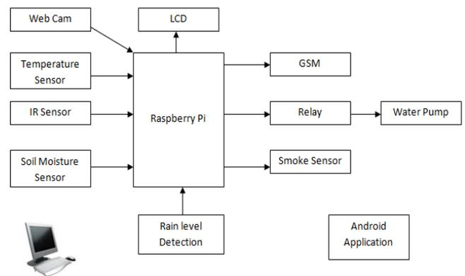
Fig 1:Block diagram of Automated Irrigation System
