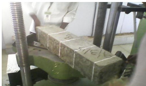
Fig 4: Testing of Beam
