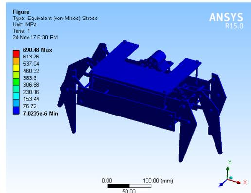
Fig -6: Von misses stress in geometry of six leg moving mechanism
