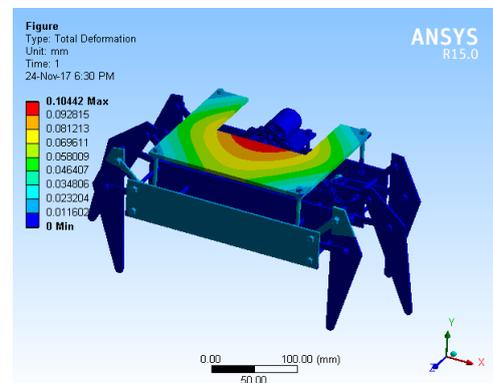
Fig -7: Displacement in Six leg moving mechanism
