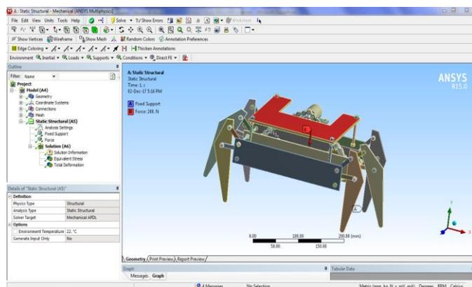
Fig -5: Boundary conditions assigned to the geometry of six leg moving mechanism
