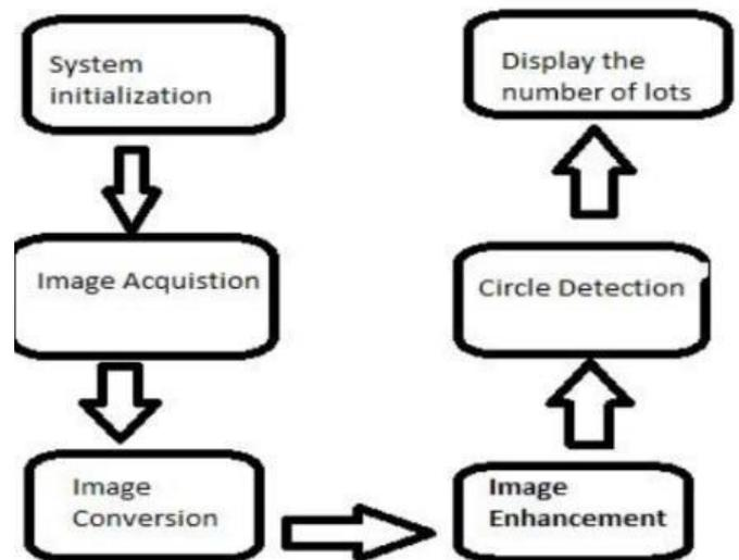
Figure 1: The process flowchart
