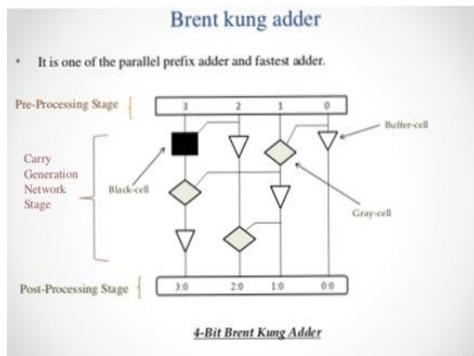
Fig: 4-bits Brent Kung adder
