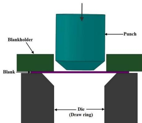
**Fig-1:** Diagram of Blanking Machine
