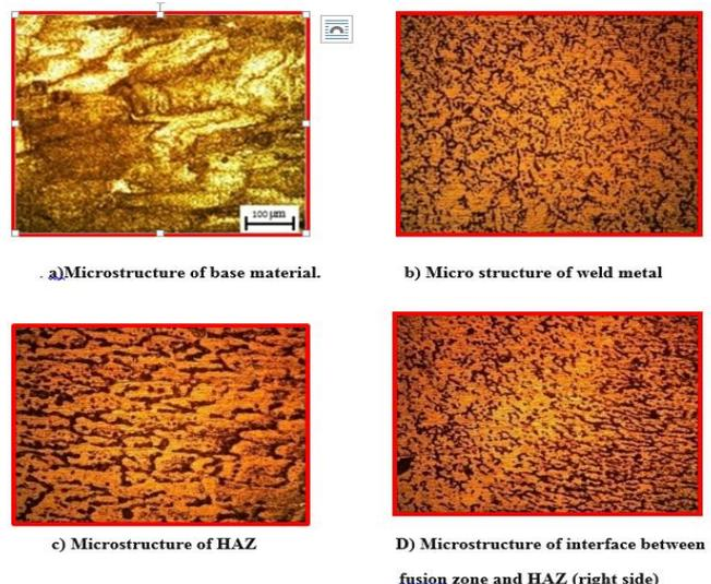
Figure 5.1- Microstructure
