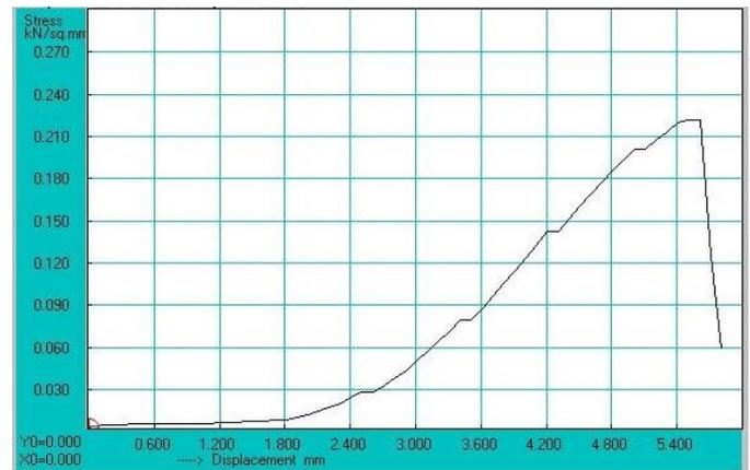
**Chart 5.3.2-** tensile test for welded material
