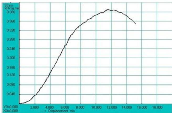
**Chart 5.3.1-** Tensile test for base material
