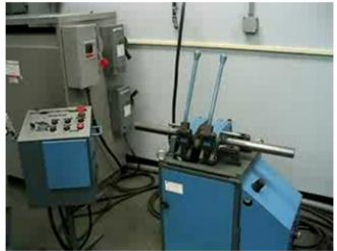
Figure - 3 : MIAB welding machine, curtesy of JIT engineering, Singapore.
