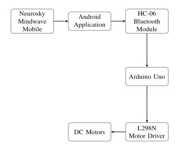
Fig -1: Hardware System Flow
