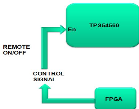
FIG 3.1 Block Diagram of Remote On/Off
