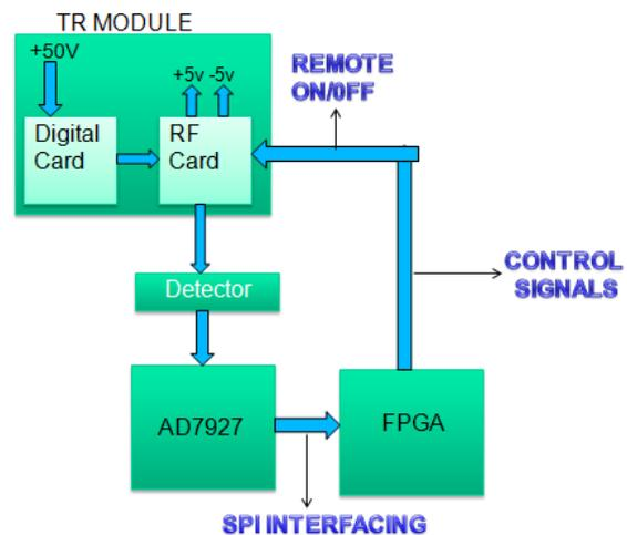
Fig 1 .1 Block Diagram of TR modules with SPI interfacing
