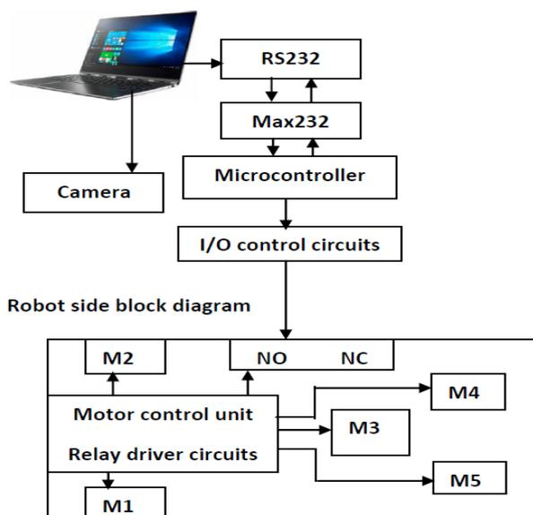
Fig -2: Block Diagram of system design for Object Pick And Place using Machine Vision System
