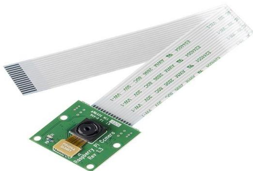
Figure3.2: Raspberry pi camera module
