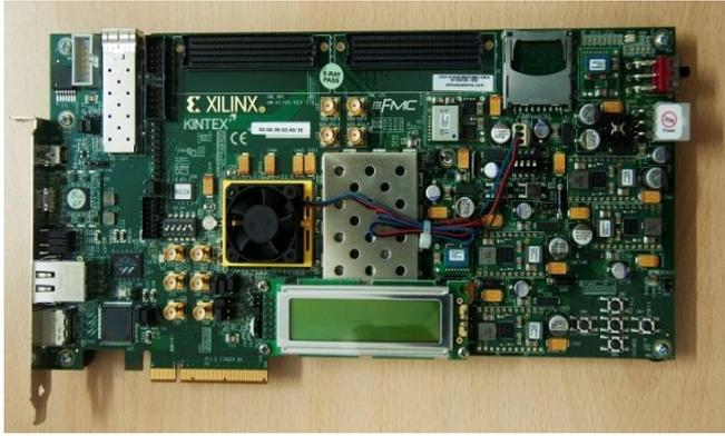
**Fig -2: Kintex-7 System Board**
