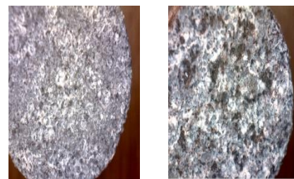
Fig 4: Optical image of AZ91+Ca+Sn Alloy after corrosion Test
