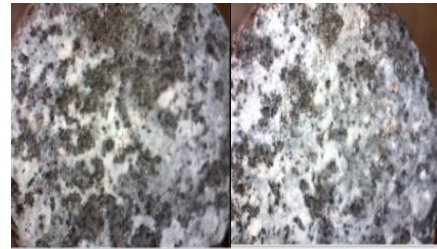
Fig 3: Optical image of AZ91 Alloy after corrosion Test
