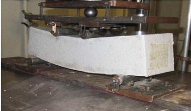
Figure 4: Flexural strength of beams
