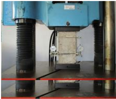
Figure 6 modulus of elasticity test
