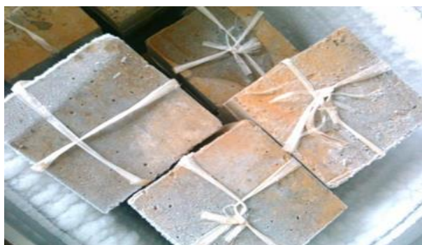
Figure 7. Freezing-thawing of crumb rubber concrete
