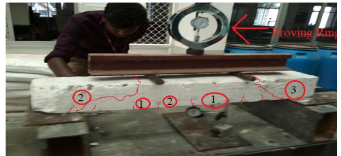
Figure 9. Experimental result structural cracks in the beam
