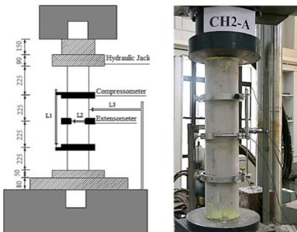
Fig. 3 Test setup (dimensions in mm)( Hanan Suliman Al-Nimry et al (2017))
