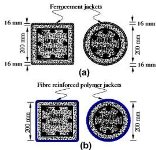
Fig-2. Arrangement of reinforcing bars: (a) ferrocement jacketed columns and (b) FRP jacketed columns (M. Yaqub et. al (2013))
