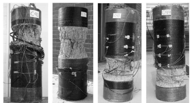
Fig -1 :Rupture aspect of RC columns confined with 1,2,3 and 4 CFRP layers (Carlos Chastre and Manuel A.G. Silva (2010)
