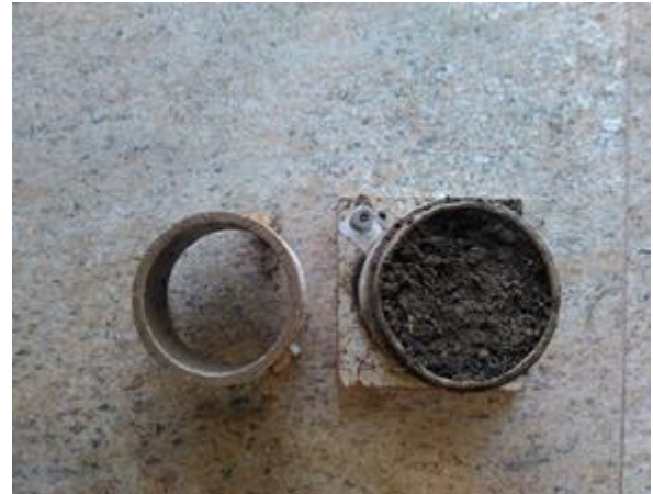
Figure - 5 Standard proctor apparatus
