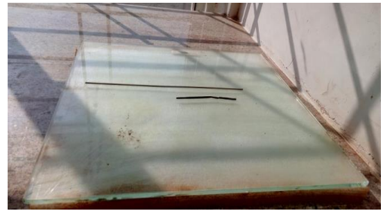
Figure - 2 Plastic limit
