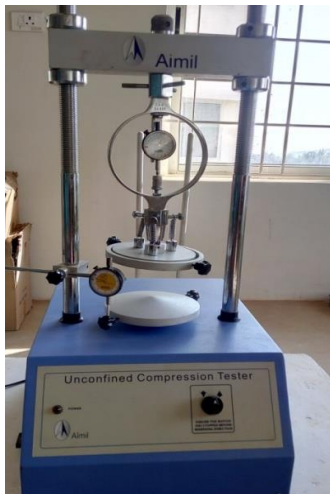
Figure - 3 UCS testing apparatus
