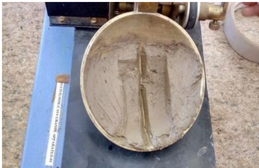
Figure - 1 Liquid limit
