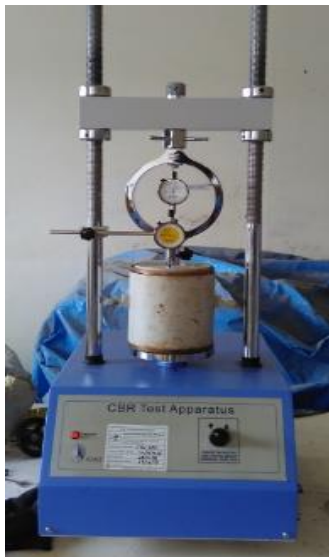
Figure - 6 CBR apparatus
