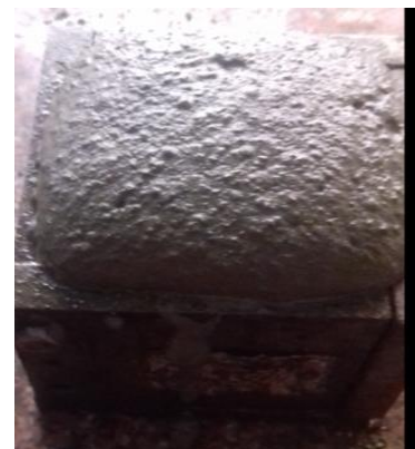
Fig 3 – Aerated specimen 30 minutes after casting
