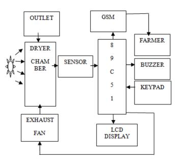
Figure-4:Circuit Diagram of Solar Dryer
