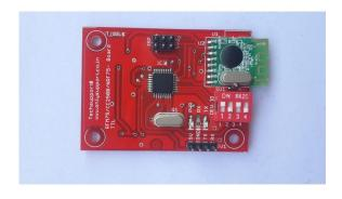
Figure 6.1.2 Zigbee Structure
