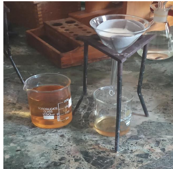
Fig-2: Filtration of final Neem Bio-oil
