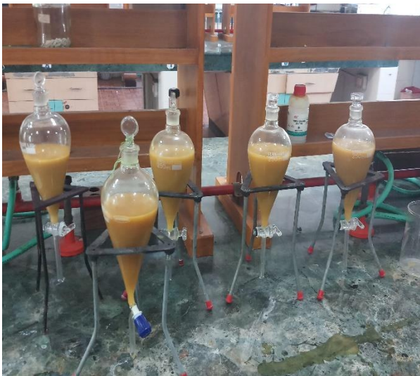
Fig-1: Separation of Neem Bio-oil
