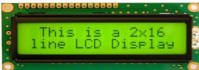
**Fig 5: LCD Display**
