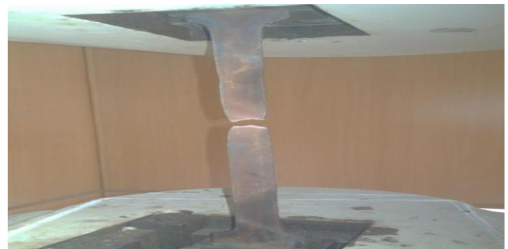
Fig.1.3 Breakage point of coupon test specimen at ultimate load
