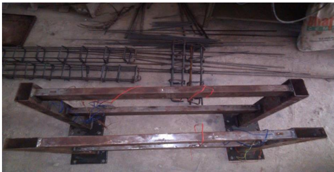
Fig.1.5 (b) Frames along major and minor axis
