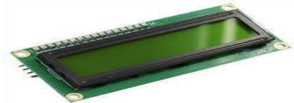
Fig:5.2. 16x2 LCD Display
