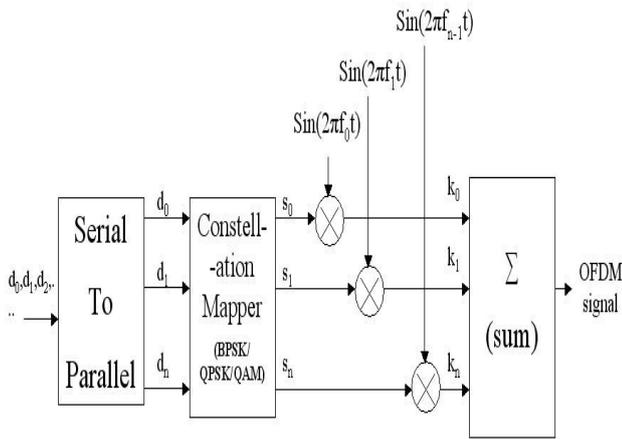
FIG-1: OFDM transmitter
