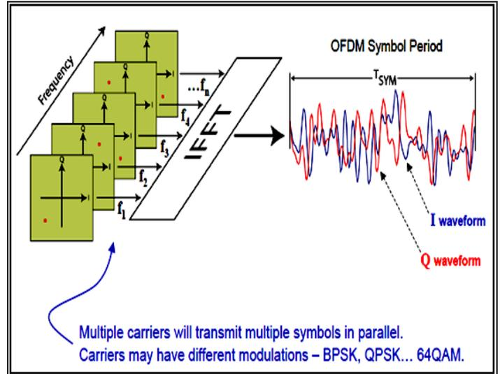
OFDM transmission using BPSK modulation technique
