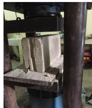
Figure - 2: Failure mode of concrete block after loading.
