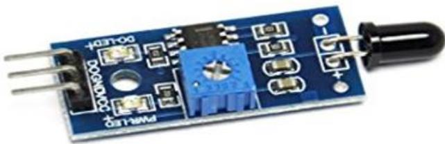
Fig -5: Flame Sensor Module
