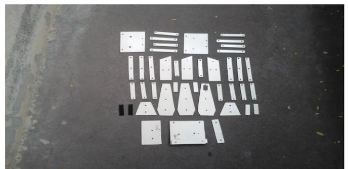
Fig -1: Mica pieces after cutting and drilling
