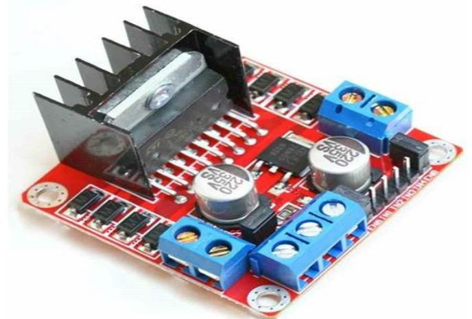
Fig -4: Motor Driver ST L298N (5 Amps Peak)
