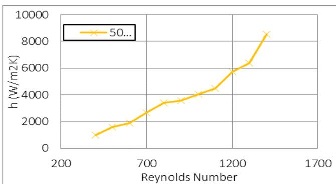
Fig -4: Heat transfer coefficient Vs Reynolds number, with oil for 50° corrugation angle.
