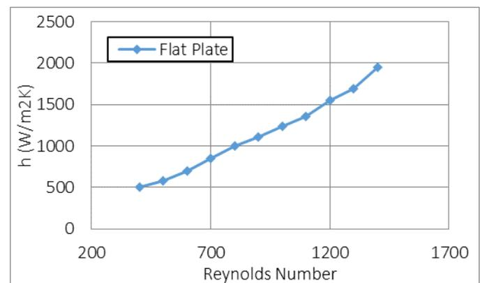
**Fig. -1: Heat transfer coefficient Vs Reynolds number, with oil for flat plate.**
