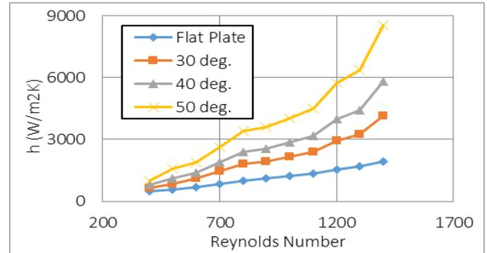
Fig -5: Heat transfer coefficient Vs Reynolds number, with oil for flat, 30°, 40° and 50° corrugation angle
