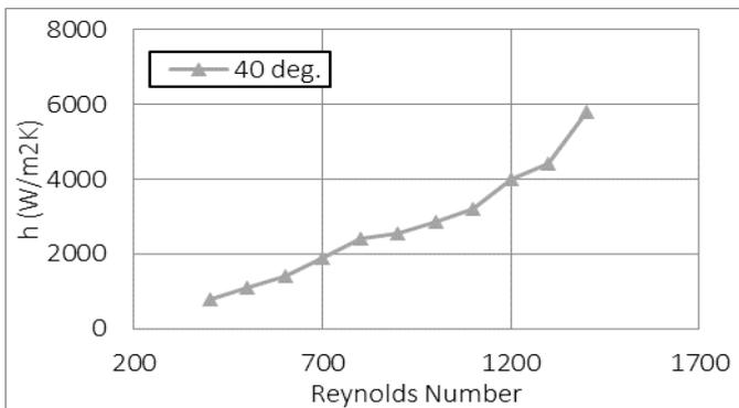
Fig -3: Heat transfer coefficient Vs Reynolds number, with oil for 40° corrugation angle
