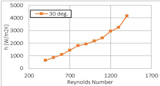
Fig -2: Heat transfer coefficient Vs Reynolds number, with oil for 30° corrugation angle
