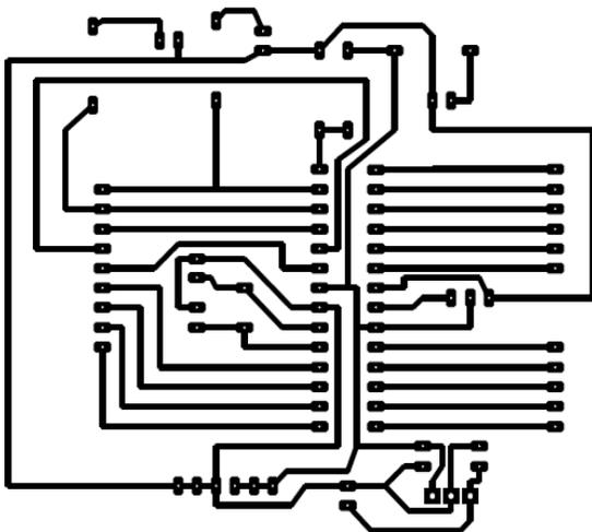
Fig.3 ARDUINO copper
