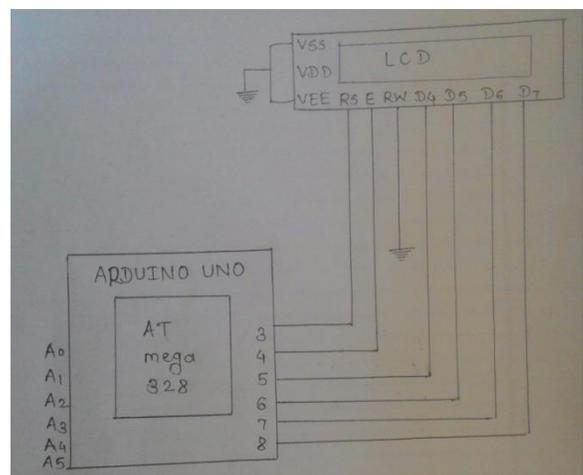
Fig.5 LCD ARDUINO interfacing diagram
