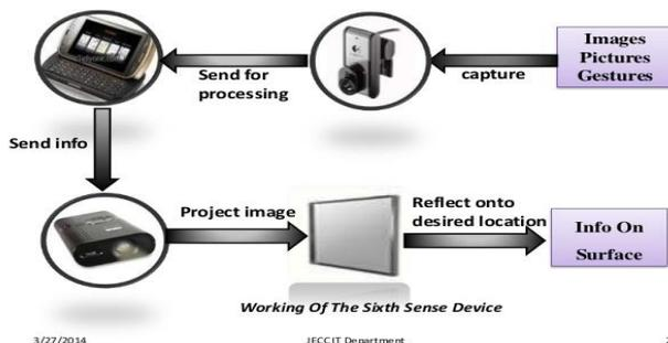
Figure 5. Working of Sixth Sense Device
