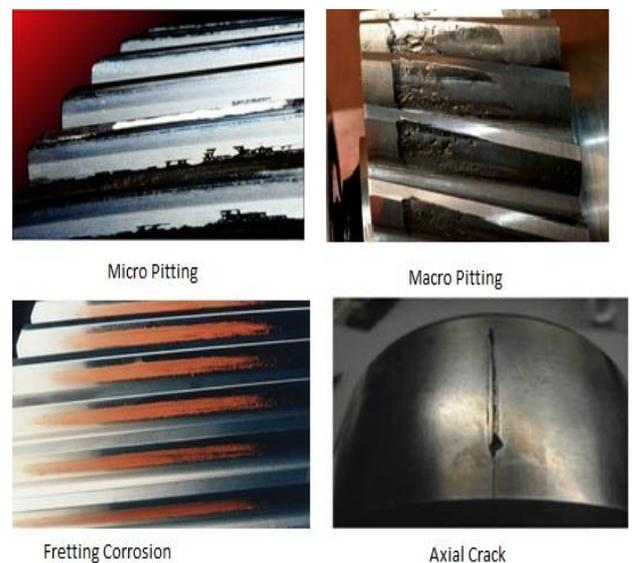
Figure.3 Failure due to load
