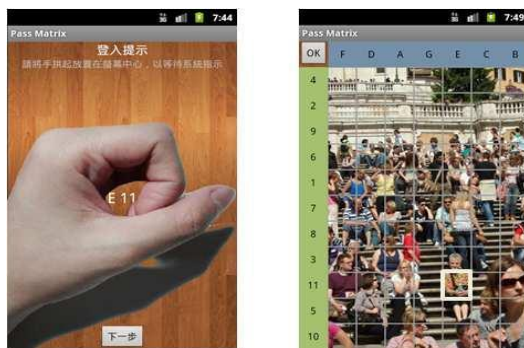
Fig. 7. (a) Get the login pointer (E,11) straightforwardly. (b) Get the login marker through a predefined picture.
