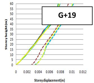
Fig 5 Maximum storey displacement with storey height
