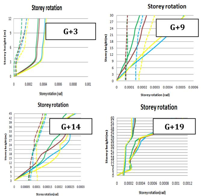
**Fig 3** Maximum storey rotation with storey height
