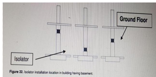
Figure 22. Isolator installation location in building having basement.
