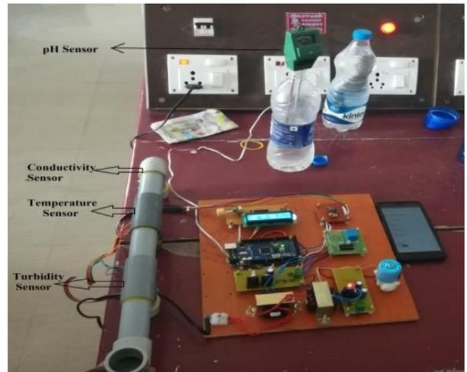
**Fig -1:** The picture shows the water quality monitoring using Wi-Fi module
