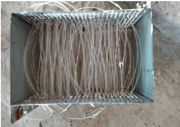
Fig -1: Optical fibers arranged in the mould
