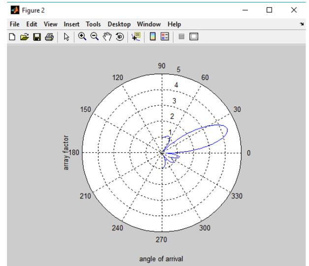
Fig- 6:polar plot of smart antenna
