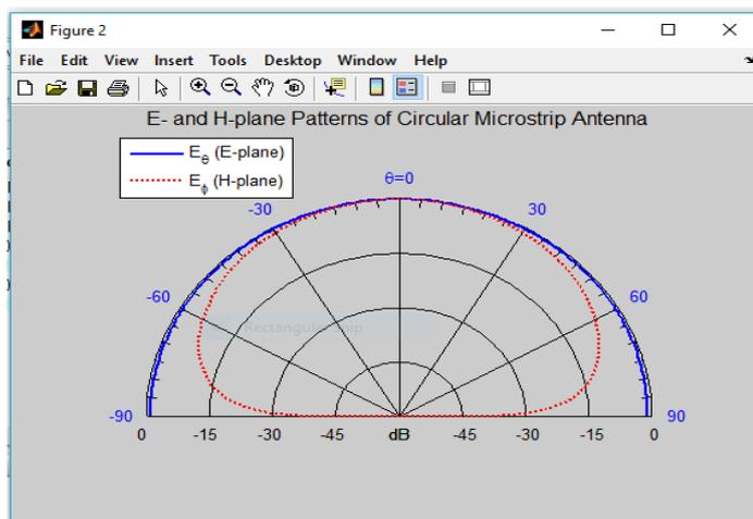
Fig-4: radiation pattern of circular patch antenna
