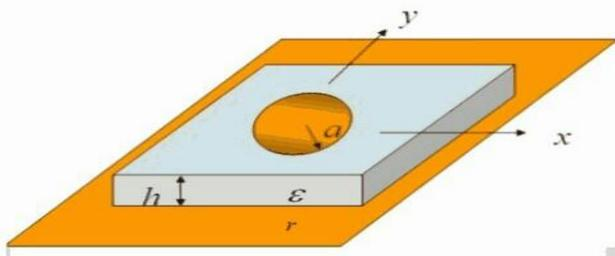
Fig-3: circular patch antenna
