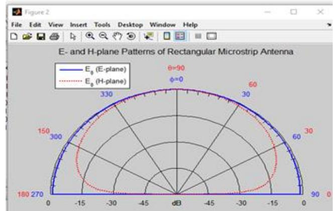
Fig-2: radiation pattern of rectangular patch
