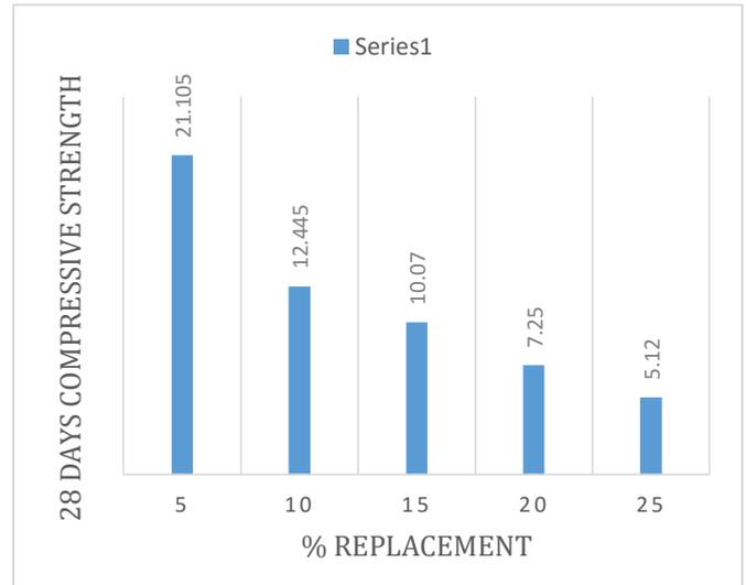
**Fig-2:** Compressive strength comparison for cubes
