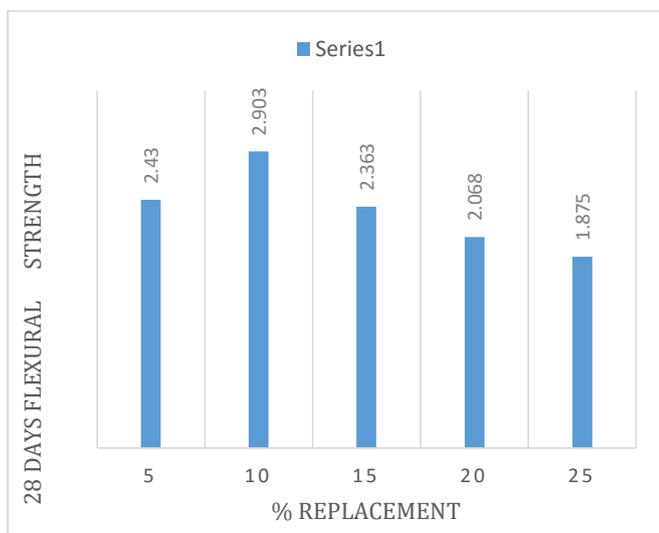
**Fig-4:** Flexural strength comparison for beams
