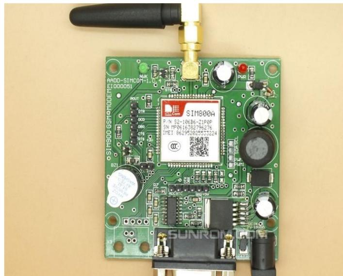
**Fig (3) GSM Module**
