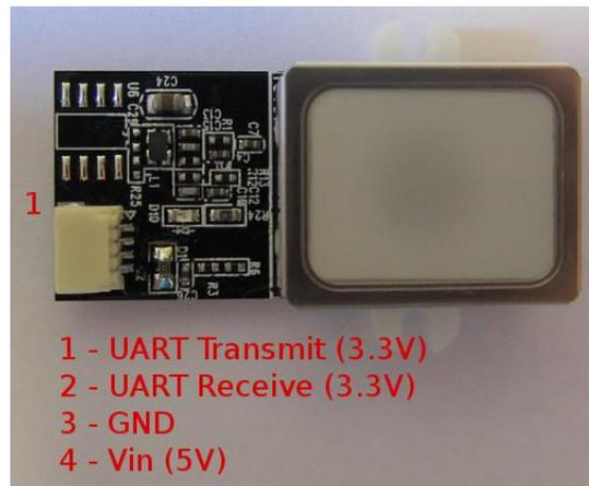
Fig (2) Fingerprint Module
