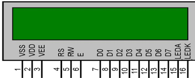
Fig (4) LCD Display
