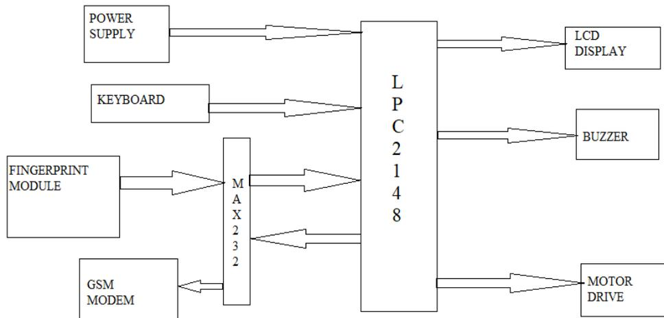
Fig (1) Block Diagram of LPC2148
