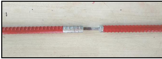
Fig-10: By Interference fit method
