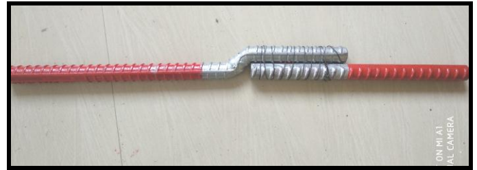
Fig-16: By binding wire method
