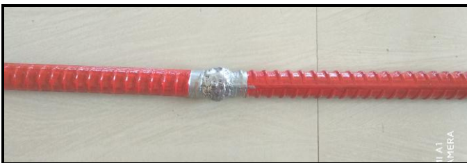
Fig-13: By welding joint
