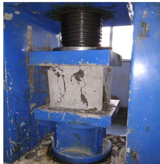
Fig -1: Compressive strength Test
