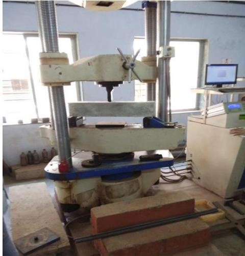
Fig -2: Flexural strength Test
