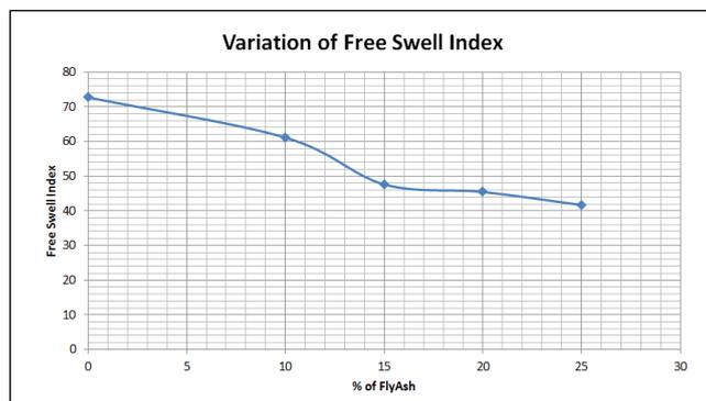
It is observed that with the increase in percentage of fly ash free swell values are decreasing. This is due to decrease of the amount of repulsion between clay particles due to replacement of clay by fly ash particles.
