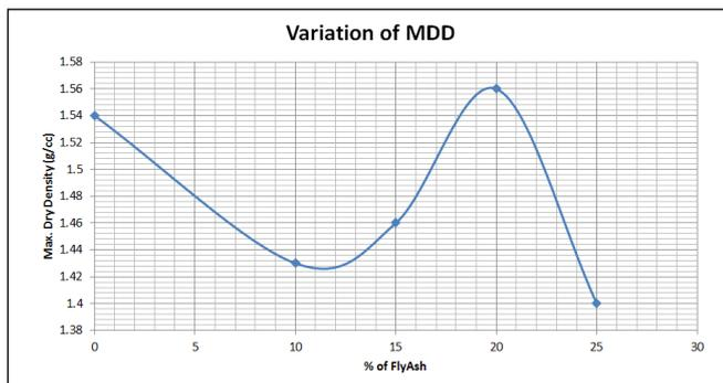
From the compaction test data it is identified that with increasing the percentage of fly ash, MDD values are varying abruptly. Low dry densities are due to nature and low specific gravity of fly ash particles compared to clay particles. As the percentage of fly ash is increased, soil particles get oriented and hence dry density increases.
