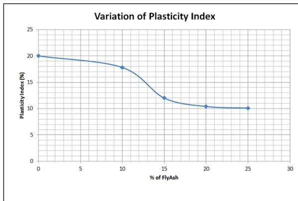
From the consistency test data, it is identified that as the percentage of fly ash is increasing plasticity index values are decreasing. This is due to the decrease in diffused double layer by replacement of clay particles by fly ash particles and also due to the development of shear resistance at the inter particle level.
