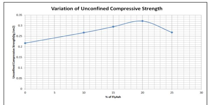
From UCC test, it is observed that unconfined compressive strength increases with increase in fly ash content .As the clay particles are replaced by fly ash, strength increased and it can take more load. Beyond the optimum percentage of fly ash, UCS decreased.
