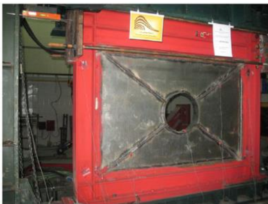
Fig - 6: Special perforated diagonally stiffened specimen (Alavi et al. 2013)
