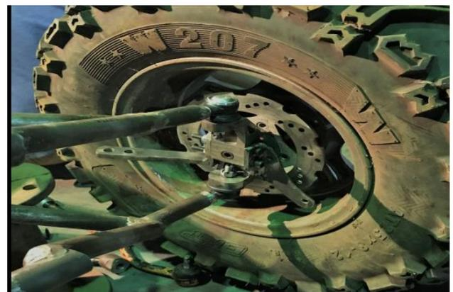
Fig. 4. Actual image of Modified knuckle.
