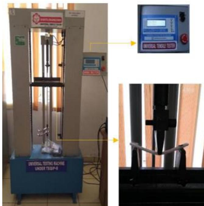
Fig. 5 Flexural testing in Universal Tensile Testing Machine
