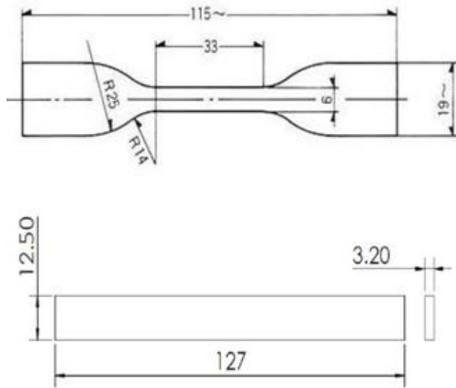
Figure 1. ASTM standard sample for Tensile and flexural testing (dimensions in mm)
