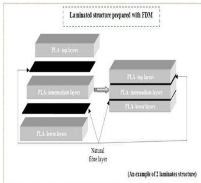
Figure 2. Layering and embedding process to develop samples
