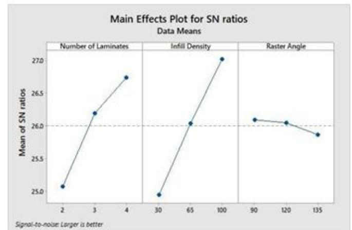
Fig. 6 Trends for the flexural Strength
