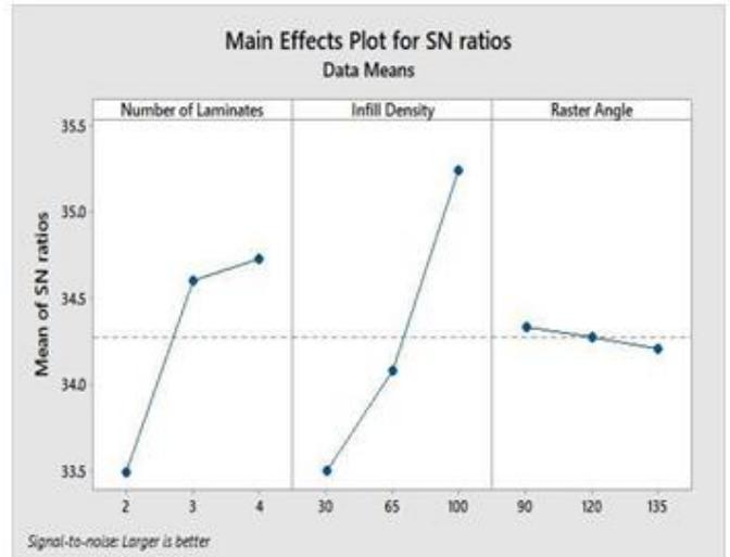
Fig. 4 Trends for the Tensile Strength
