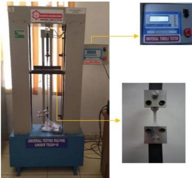
Fig. 3 Tensile testing in Universal Tensile Testing Machine
