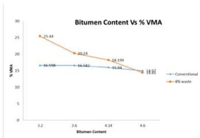
Fig No. 6 Graph of % Bitumen Vs VMA
