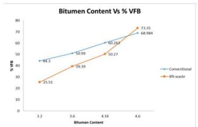
**Fig No. 4** Graph Of % Bitumen Vs Vfb
