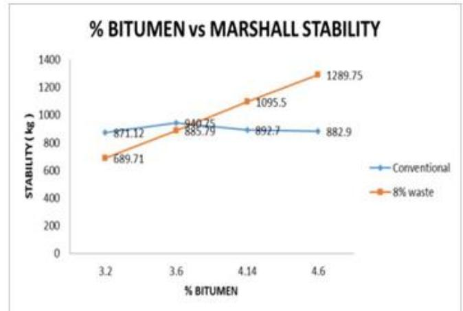
**Fig No. 2** Graph of % Bitumen Vs Marshall Stability
