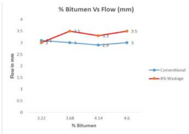
Fig No. 5 Graph of % Bitumen Vs Flow
