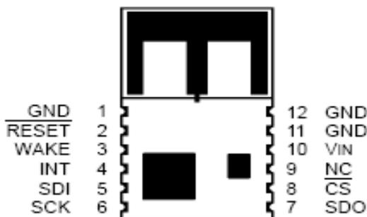
Fig-1: Zigbee pin configuration
