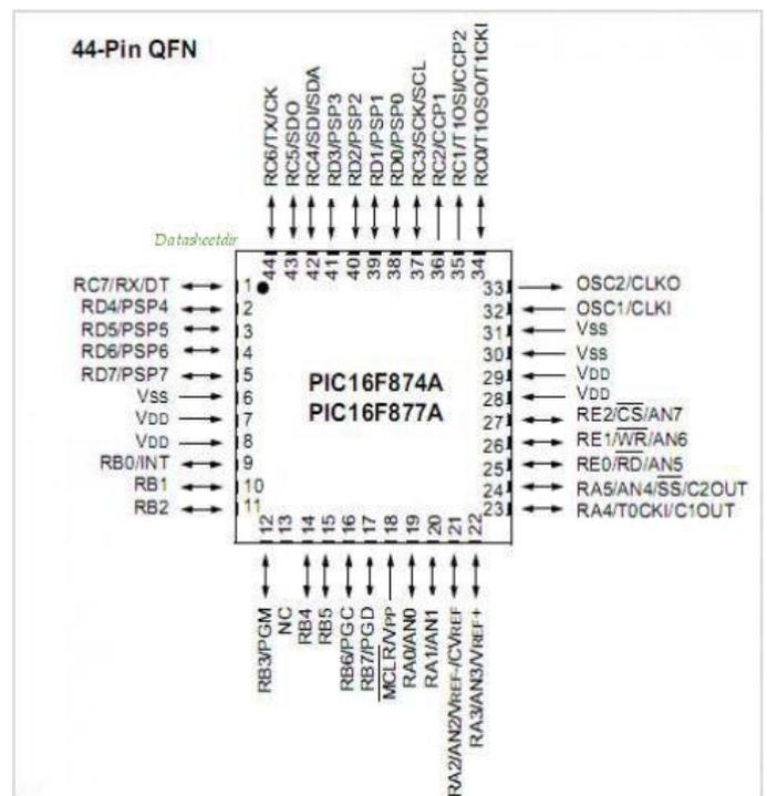
Fig-3: Microcontroller configuration
