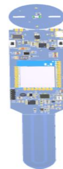
Figure 6: 3D view of hardware PCB module of sensor node.
