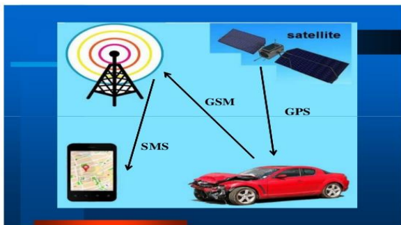
Figure no.1.1 Accident identifier using GPS & GSM
